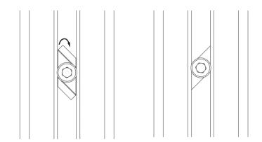
Positioning the rhombus nut by turning it clockwise
